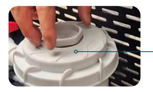
After replacing the filter element. Screw on the filter cover, open the ball valves. Then open the exhaust valve slightly to ensure there are no air locks. After this you can turn the lce bath back on
